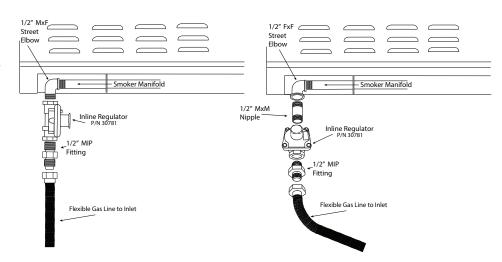
Never run flex hose behind the firebox, run the hose at an angle, straight down, or out of the back.
