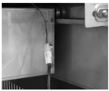
Power Supply Connection (behind rear panel) CARE & USE/INSTALLATION | 23
